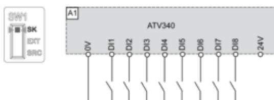
Switch Set to EXT Position Using an External Power Supply for the DI
