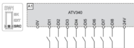
Switch Set to SRC (Source) Position and Use of an External Power Supply for the DI
