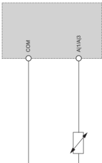
**Control Block Wiring Diagram**
