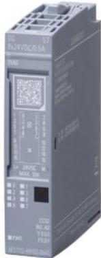
SIMATIC ET 200SP, Digital output module, DQ 8x 24V DC/0,5A Standard, Source output (PNP,P-switching) Packing unit: 1 piece, fits to BU-type A0, Colour Code CC02, substitute value output, module diagnostics for: short-circuit to L+ and ground, wire break, supply voltage
