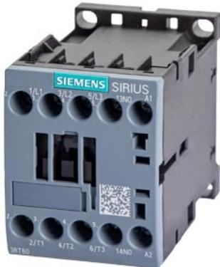
Contactor AC 230 V 50/60 HZ AC3 7.5 kW 400 V AUX contacts 1 NO 3-pole, size S00 screw terminal
