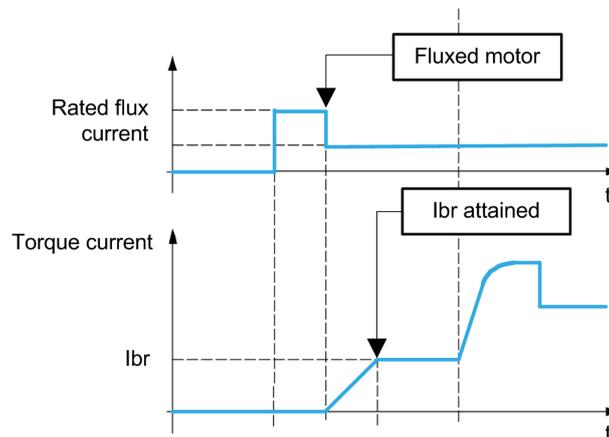
When run command is given, the drive over-fluxes the motor during a short time in order to generate a sufficient motor torque. The level of the torque is set with the parameter **[Brk Release Current]** *IBR*. This torque is required to maintain the load during the release of the brake and before starting speed control.
