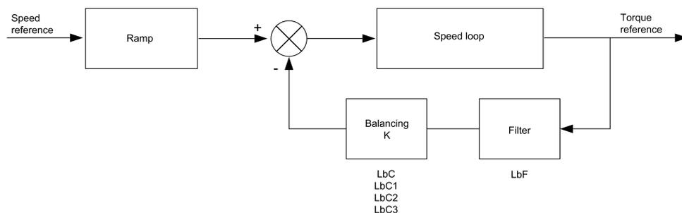
The load sharing factor K is determined by the torque and speed, with two factors K1 and K2 ( $K = K1 \times K2$ ).
