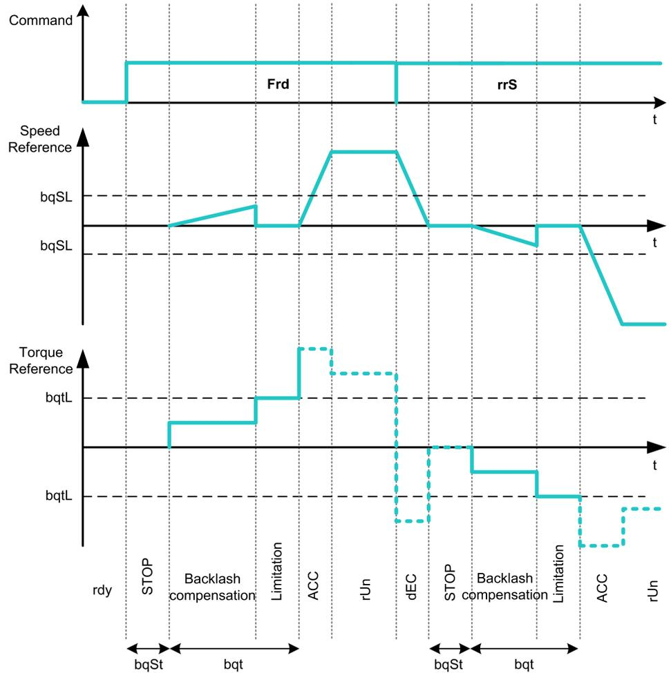
**Regulate 0Hz speed at direction change (UC-3)**
