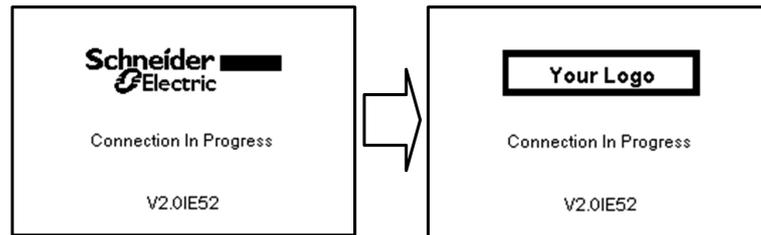
From the firmware version V2.0 of the Graphic Display Terminal, the logo displayed at power on by the Graphic Display Terminal can be customized. By default, the Schneider-Electric logo is displayed.
