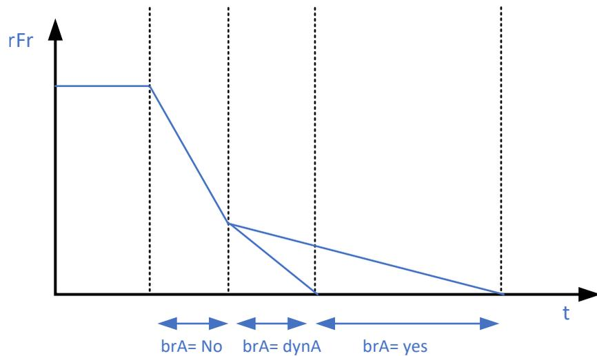
Activating this function automatically adapts the deceleration ramp, if this has been set at a too low value according to the inertia of the load, which can cause an overvoltage detected error.
