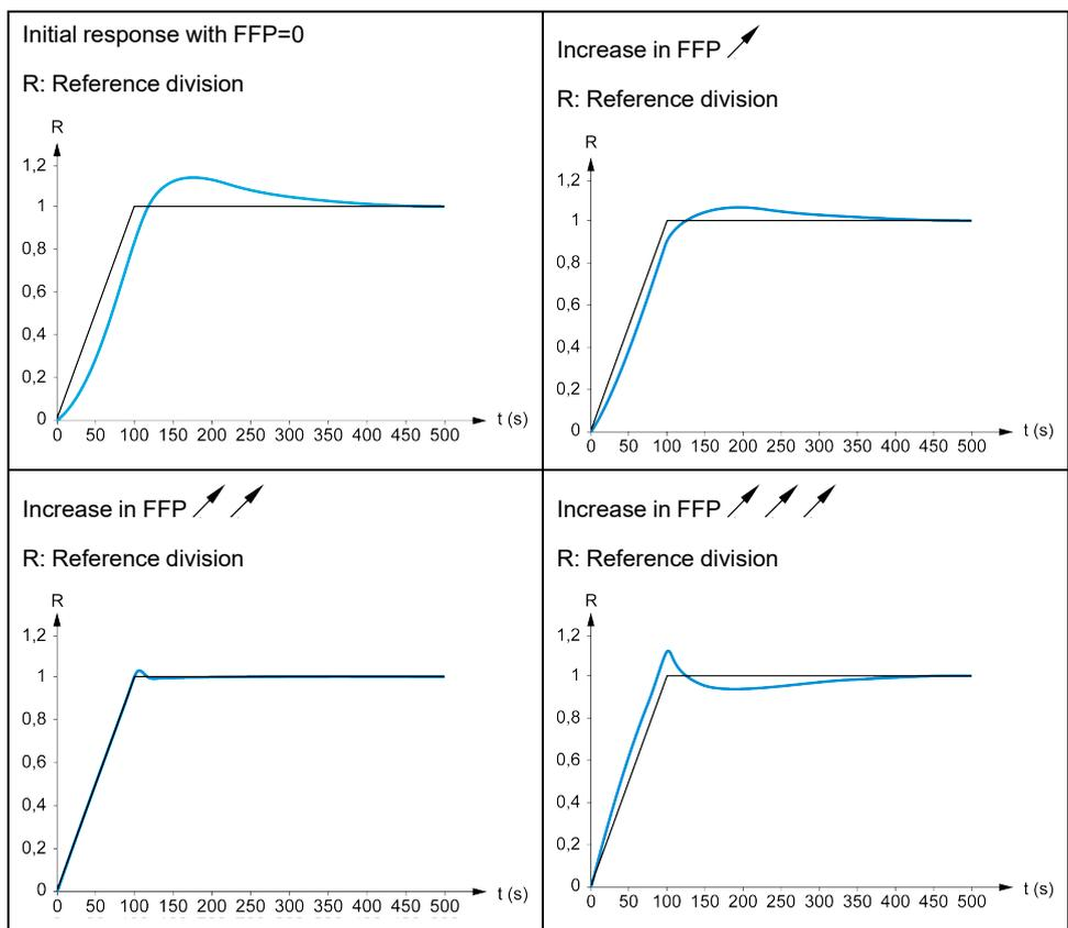
**High-Performance Speed Loop - Setting the [FeedFwd Bandwidth] FfV Parameter**
