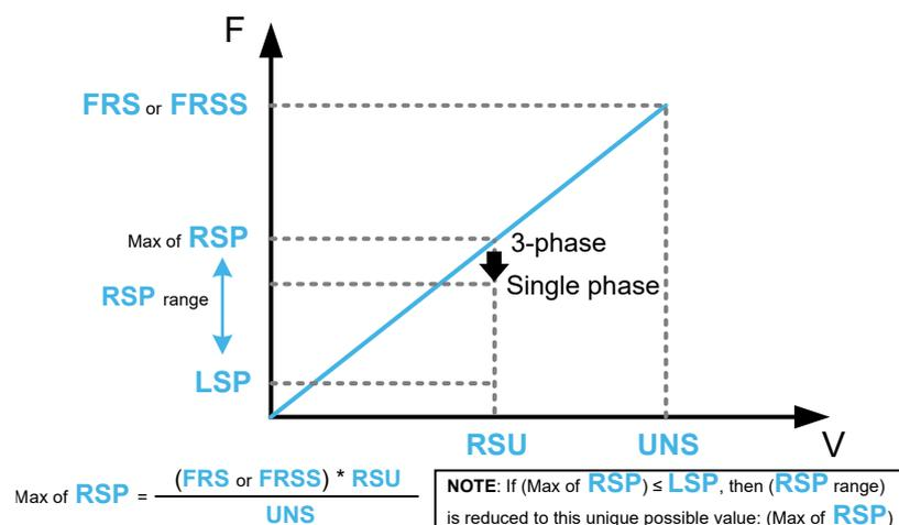
**NOTE:** Compared to a 3-phase power backup supply, the [Pwr Backup Ref Freq] RSP value may need to be reduced in order to provide the nominal torque with a single phase power backup supply. For more information, you must refer to the application note "Power Backup".
