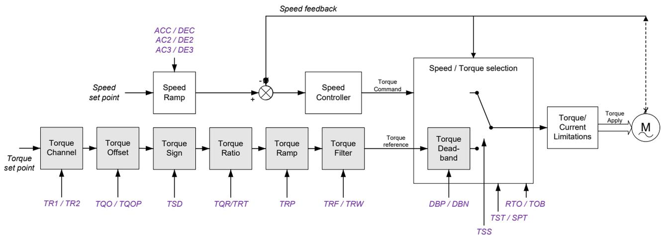
The function can be used to switch between operation in speed regulation mode and operation in torque control mode.
