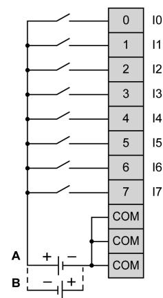
The 3 COM terminals are connected internally.
