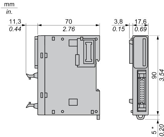
\* 8.5 mm (0.33 in) when the clamp is pulled out.
