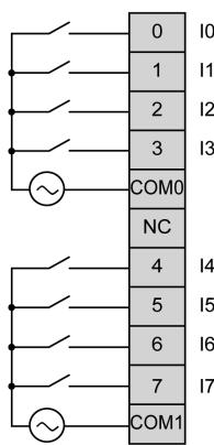
The COM0 and COM1 terminals are **not** connected internally.
