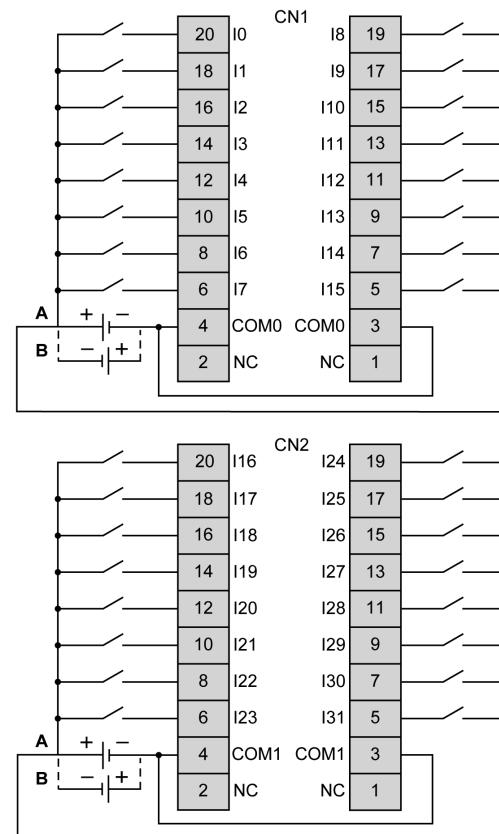
The COM0 terminals are connected internally
