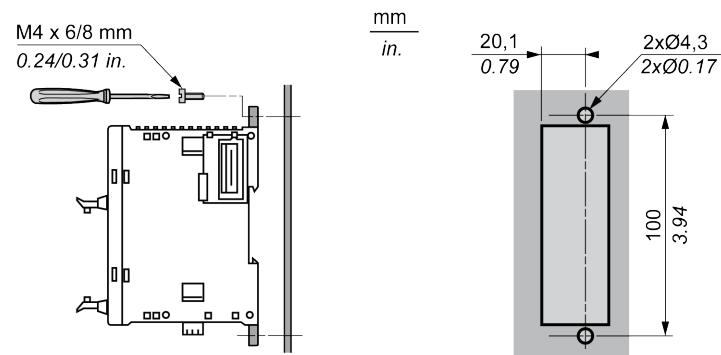
The following diagram shows the mounting hole layout for the TM3DM32R expansion module:
