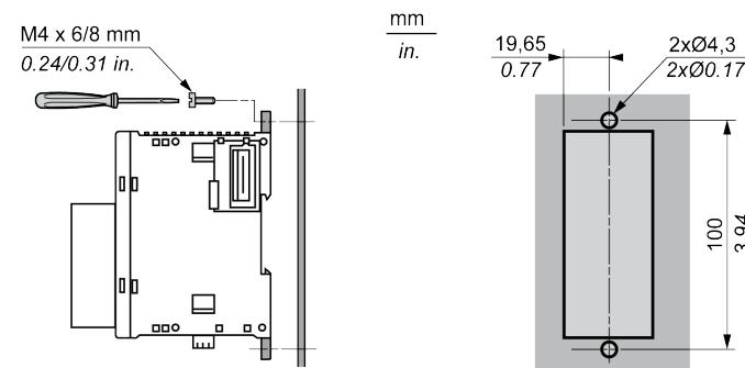
The following diagram shows the mounting hole layout for TM3 with 32 HE10 (MIL 20) I/O channels:
