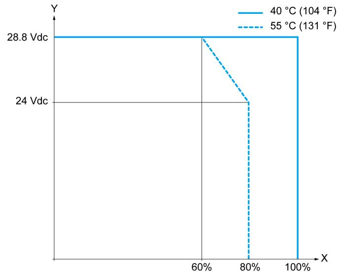
At an ambient temperature of 55 °C (131 °F) in the horizontal mounting direction, limit the inputs and outputs, respectively, which turn on simultaneously as indicated by the X axis.
