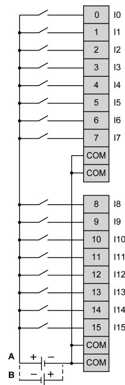
The 4 COM terminals are connected internally
