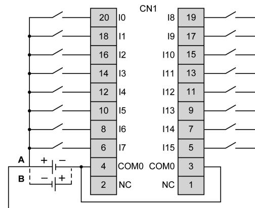
The COM0 terminals are connected internally
